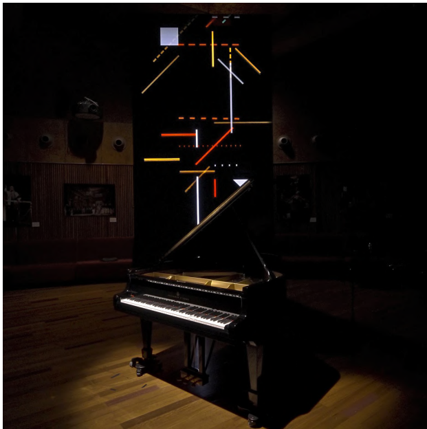
Figure 21: An image of the ppff setup in Barcelona's Liceu Opera. A vertical LED screen display the downwards scrolling scores. When the graphics arrive at the piano position they are converted into MIDI to control a Steinway&Sons Spirio grand piano.
